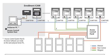
The configuration above illustrates the iCAM 7 connected to a conventional Card Access System, Many operational variations are available
